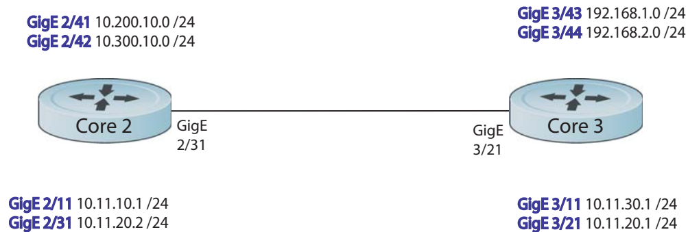
Figure 42-7. RIP Topology Example
