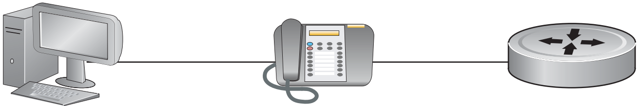
Figure 36-7. Office VOIP Deployment
